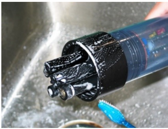
Figure 2 - Rinsing a HyQual multiprobe
