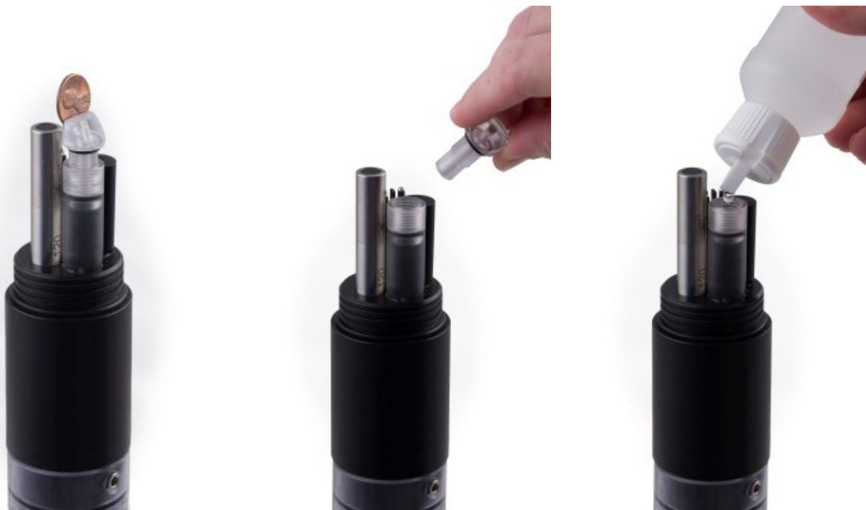
Figure 4 - Filling in fresh pH reference electrolyte
